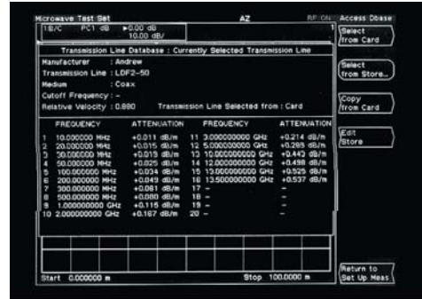
The Transmission Line Database contains the key parameters of the most common transmission lines
