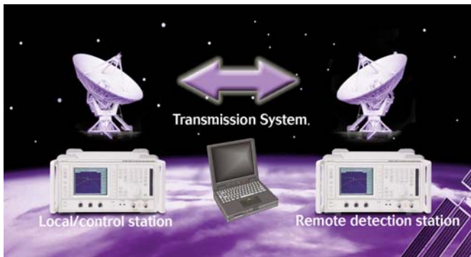
A unique measurement system designed to evaluate the group delay and in band performance over a satellite telecommunications link
