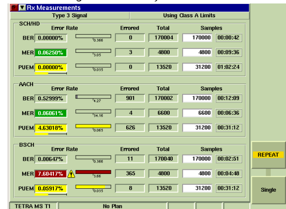
Figure 6 - Measuring receiver sensitivity using 'T1' RF loopback in the TETRA MS T1 system
